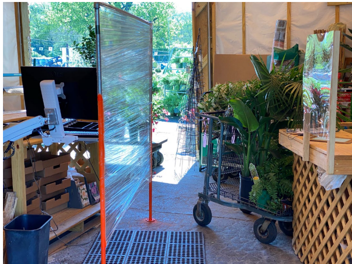
Figure 5. An inexpensive frame and shrink wrap can be used to create a barrier. Photo Credit: David Bates, Bates Nursery and Garden Center
