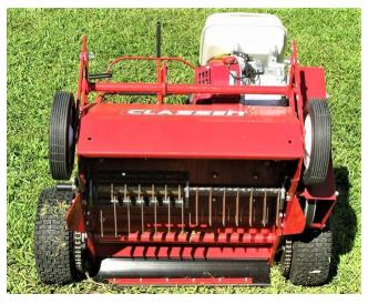
*Walk-behind mechanical dethatchers are engineered to slice into the lawn and lift thatch.*
