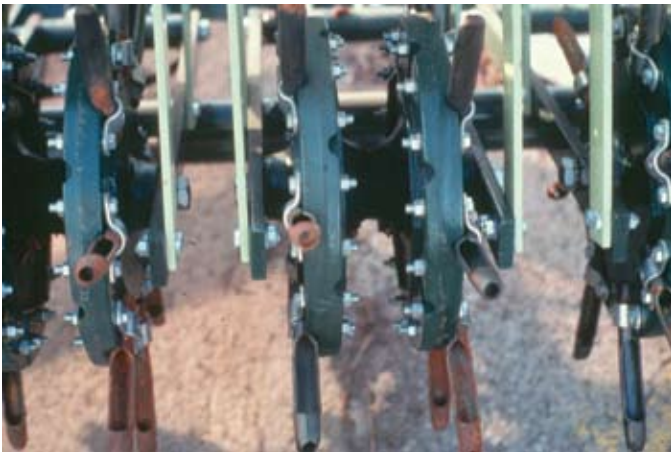
Figure 6. A rotary-motion, hollow-tine core aerifier.
