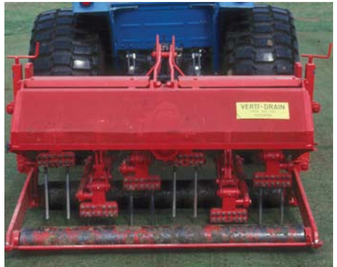
Figure 7. A deep-tine core aerifier.
