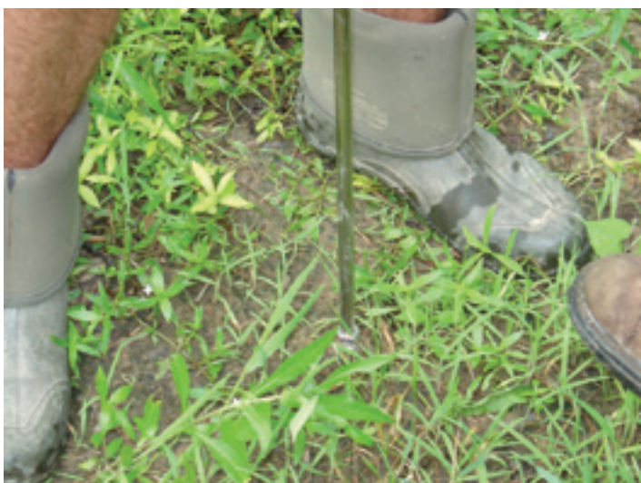
Figure 6. A soil probe was used to extract a soil core at each plot center
