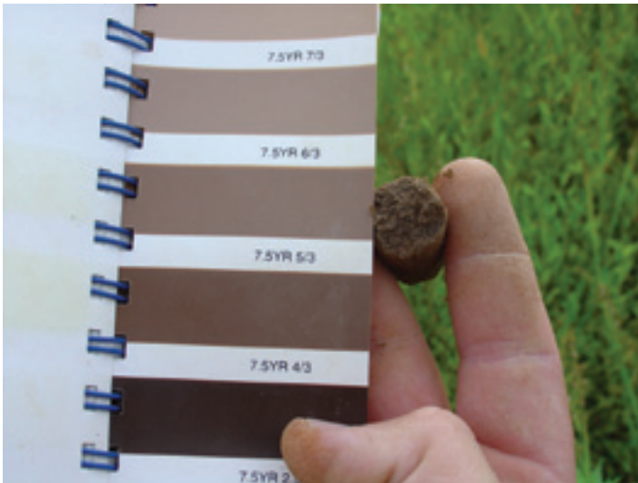
Figure 8. The soil core shown corresponds to a Hue of 7.5 YR, Value 5 and Chroma 3, which has no gray mottles.
