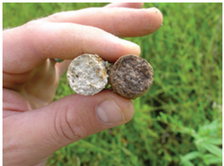
Figure 11. These cores contrast poorly drained (left, 95 percent gray) with well-drained (right, zero percent gray) soils.
