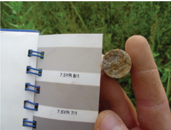
Figure 10. The soil core shown is approximately 50 percent gray, indicating poor drainage and that the gray matrix has been met.
