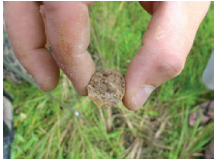
Figure 9. The soil core shown is approximately 30 percent gray, indicating some drainage impairment.
