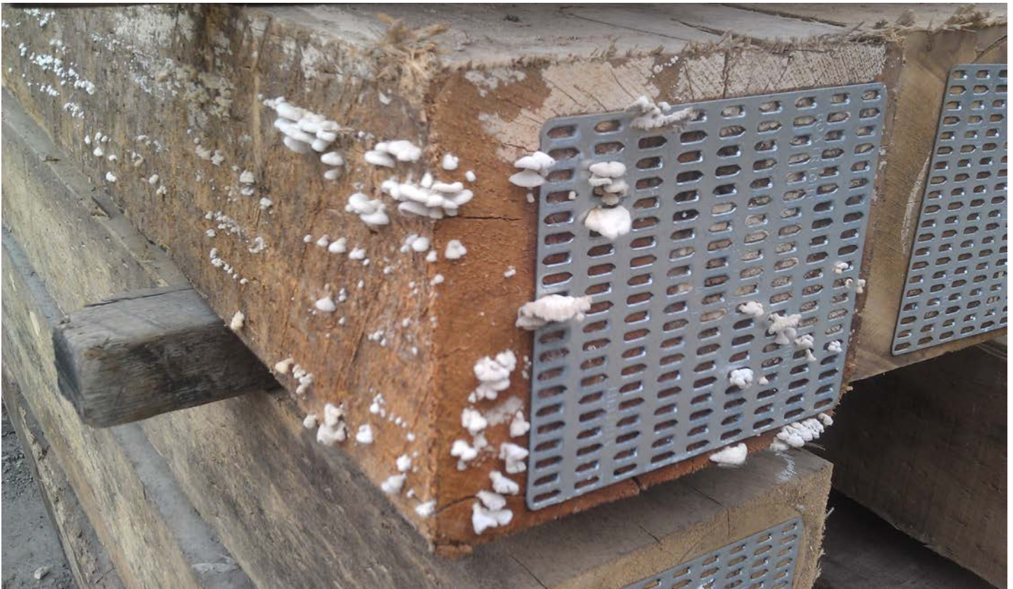
FIGURE 6. The white fungal fruiting bodies on this tie mean that rot is well-established and strength loss has occurred. Wood weight loss as low as 2 percent caused by decay can cause as much as 30 to 50 percent strength loss.
