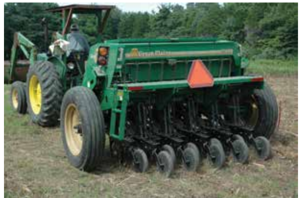
Fig 15; Drilling seed is the most efficient planting technique. Seed is planted at the proper depth, and germination rates and seedling survival are greater.
