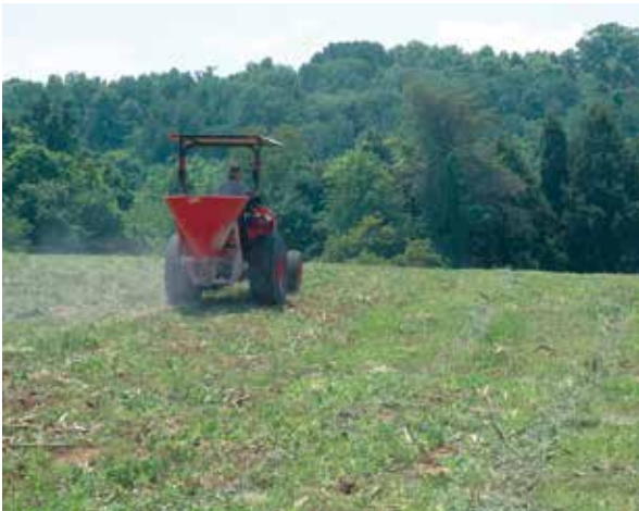
Fig 12; Fertilizer applications are most easily accomplished with a cyclone spreader. Calibrating the spreader prior to fertilizer applications is just as important as calibrating it prior to sowing seed! Here, fertilizer is being spread prior to planting a warm-season food plot.
