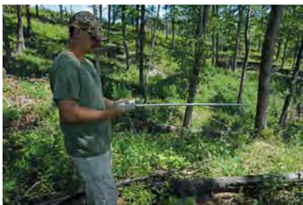
Fig 15. A ceptometer provides precise measurements of light infiltration when conducting research related to vegetation response and available sunlight. Fortunately, this level of precision is not necessary when implementing FSI.
