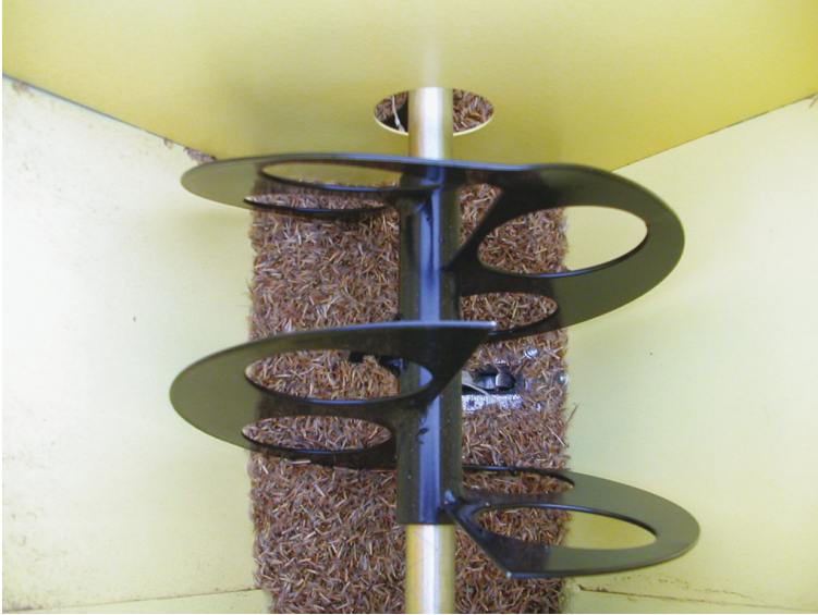
Figure 7.11. The specialized chaffy seed or “native grass” boxes on many drills include large agitators such as those on the Truax drill shown here. These agitators keep the chaffy seed from bridging and maintain an even flow through the box and cups below. Credit, D. Hancock.
