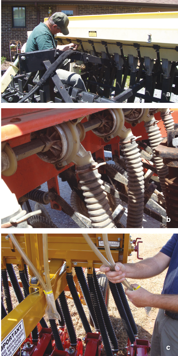
Figure 7.10. The large seed cups and straight drop tubes on the Truax (a), Tye (b) and Haybuster (c) drills shown here all allow for easy passage of native grass seed. Credit (c), K. Goddard.
