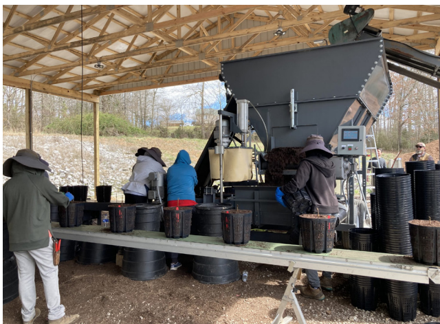
Fig. 3. Adopting a potting machine includes related investments such as a structure to house it and one or more hoppers.
