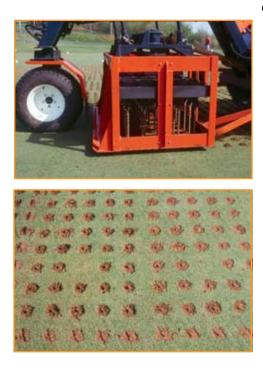
or deep-tine aerifier, the results may be well worth the additional time. As the name implies, soil is lifted to the turf surface by the drillingaction of large, hardened steel aeration bits. Bits from 1/2 to 1 or more inches in diameter and up to 16 inches in length create deep
