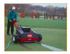
water are directed through small-diameter nozzles penetrating thatch, loosening soil and promoting root growth. Although water injection cultivation is no substitute for coring, it is often used to cultivate stressed turfs during unfavorable weather. This technology has been well-received by many golf course superintendents managing quality creeping bentgrass greens prone to hightemperature stress and wear injury during hot, dry summer months.
