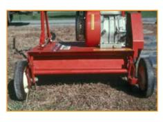
spinning, horizontal shaft may be used to relieve 'grain,' dethatch or cultivate turf. For example, grain is reduced when the knives are set to sever aboveground runners
