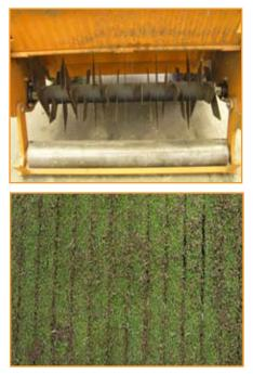
cutting blades from 3/64 to 3/8 inch thick are spaced vertically (e.g., 1 inch on center) on a shaft horizontal to the soil surface. Rows of exposed soil form as these machines move across the turf. Larger, tractordrawn linear aerators are also available. Linear aeration may expose much more of the soil surface area than core aerification.
