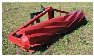
The roller crimper, with angle iron blades, crimps the stems and lays the intact plant uniformly on the ground.
