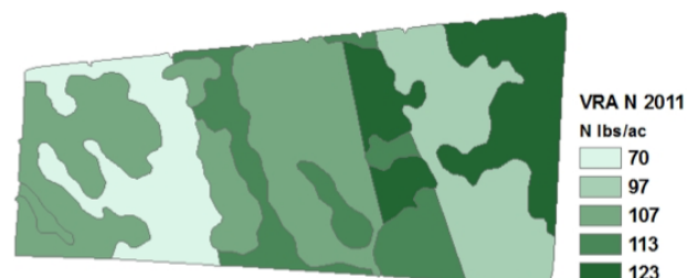
Figure 5. Variable rate (VR) nitrogen (N) prescription map for a field under zone management.
