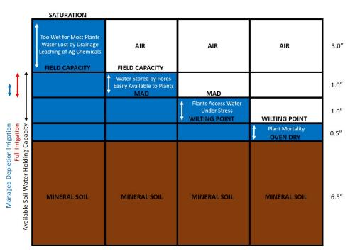
**Figure 1:** Soil Water Continuum (when air, water and soil are disassociated from pores in a 1-foot column).
