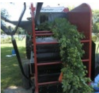
Figure 25: Small combine used to separate cones from bines.
