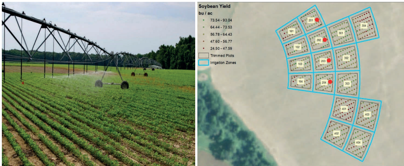
Figure 3. Irrigation zones on a VRI equipped center pivot (left) and plots layout showing yield points, trimmed plot, and water loggers/sensors station (●) areas (right) in Milan, Tennessee (2018).
