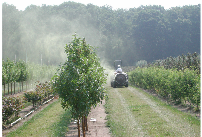
Fig. 1. Air-blast sprayers emit a large spray cloud that can lead to off-target movement of pesticides. Orchard (left), nursery (right). Photo credit: A. Fulcher, H. Zhu
