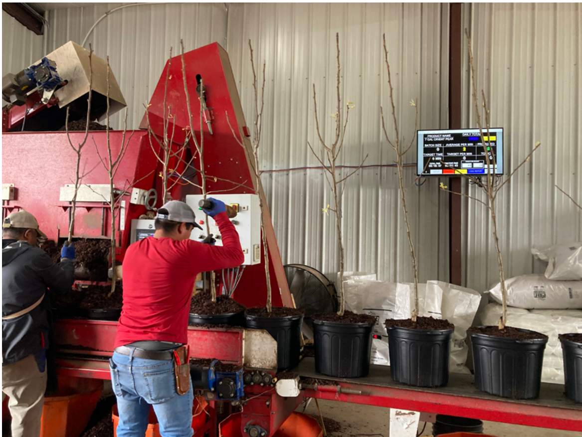
Figure 5. Inventory systems that work in conjunction with potting machines can aid nurseries in not only counting plants but also giving workers a visual reference of their progress toward daily potting goals.
