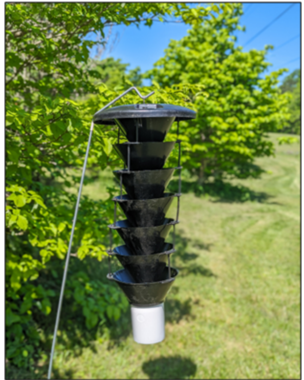
Figure 8. A Lindgren funnel trap on a 1.5 meter (4 foot) tall pole. (Image courtesy of Axel Gonzalez, PhD student, The University of Tennessee).
