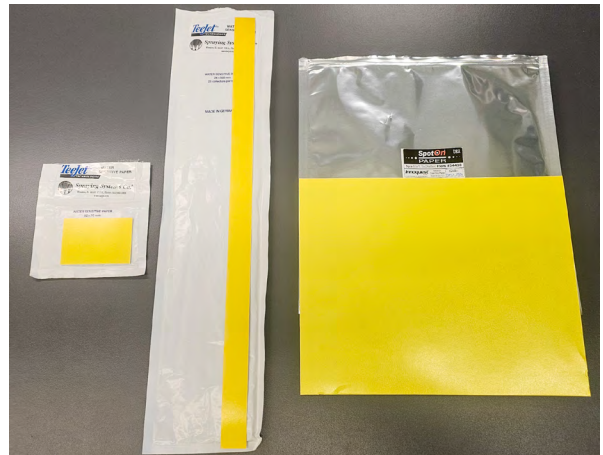
Figure 2: WSP is available in many shapes and sizes from multiple manufacturers. Each brand has slightly different characteristics. Use WSP from a single manufacturer for consistent results.
