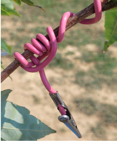
Figure 3: Growers and researchers use specialized tools and equipment such as clip assemblies (3A), boards (3D) and drift structures (3E) to distribute water sensitive paper cards (3B), strips (3C) and sheets (3F) throughout production blocks to help determine where their spray is landing.
