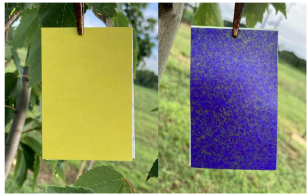
Figure 1: WSP cards change color from yellow to blue when contacted by liquid. Cards are secured to branches with clip assemblies.
