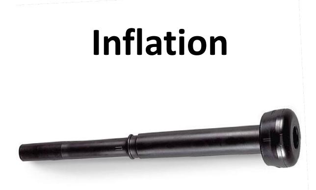
Made from flexible materials; attaches to cow's teat during milking; normally surrounded by a rigid shell
