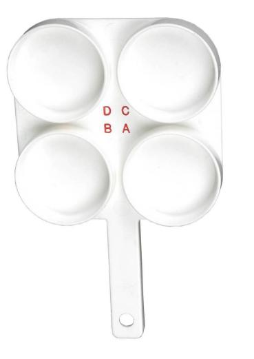
Used in mastitis detection; milk is placed into each section and a reagent is added that helps identify cases of mastitis
