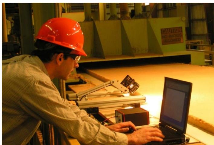
CRC researcher makes new measurements on the densification of medium-density fiberboard production for improved process monitoring and control.
